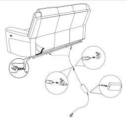
Safety Note: Transformer and cables are not to be placed under or within the recliner structure.
